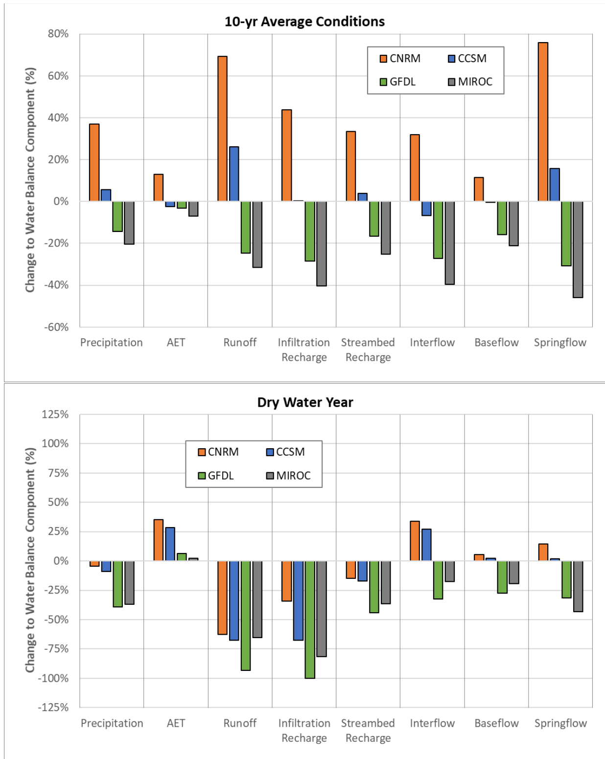
Figure E11: Percent change in various components of the water balance for the four climate change scenarios relative to existing conditions; 10-yr average conditions (top) and the driest water year in each 10-yr simulation period (bottom).
